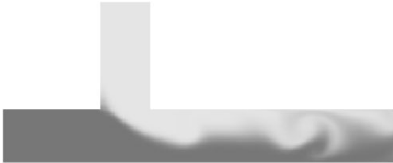
Figure 4. Instantaneous temperature fields in a 2D unsteady Tee junction at t = 12.2 s (8 recirculation times)—non-physical temperature regions (i.e. out of limits) are denoted by dark contours. Upwind; T_{\max} = 550 K – T_{\min} = 500 K.
