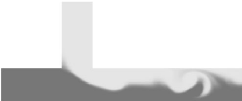
Figure 3. Instantaneous temperature fields in a 2D unsteady Tee junction at t = 12.2 s (8 recirculation times)—non-physical temperature regions (i.e. out of limits) are denoted by dark contours. Quick; T_{\max} = 550 K – T_{\min} = 500 K.
