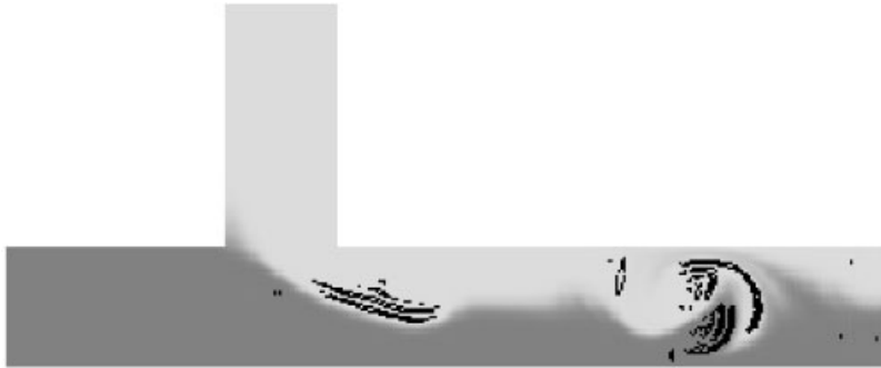
Figure 2. Instantaneous temperature fields in a 2D unsteady Tee junction at t = 12.2 s (8 recirculation times)—non-physical temperature regions (i.e. out of limits) are denoted by dark contours. Centred 4th order; T_{\max} = 554.9 K – T_{\min} = 494 K.
